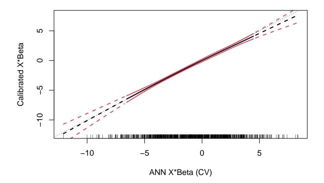
More on calibration and the calplot() function are described in the "Calibraiton of Machine Learning Models" vignette. A calibration plot for the ANN including the relaxed lasso as an offset is
