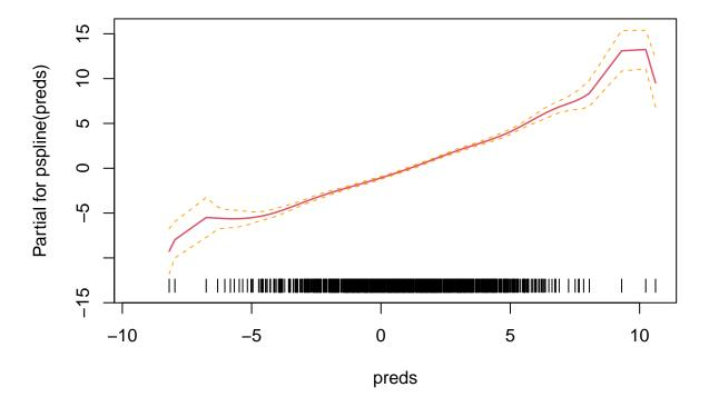
Here the linear calibration coefficient is about 1 and the spline fit on the predicteds about linear with wiggle in the extremes where there are few data.
