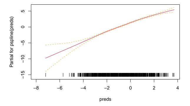
The spline fit depicted in this graph does not appear to be consistent with a stright line suggesting the NN is not, in its current form, well calibrated.
