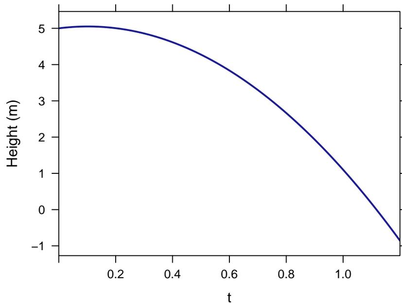
What's nice about the differential equation format is that it's easy to add features like the buoyancy of water and drag of the water. We'll do that here by changing the acceleration (the  $dv$  term) so that when  $x < 0$  the acceleration is slightly positive with a drag term proportional to  $v^2$  in the direction opposed to the motion.
