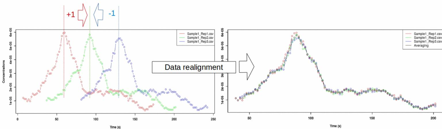
Figure 10: Sample replicate realignment and averaging in raster mode
