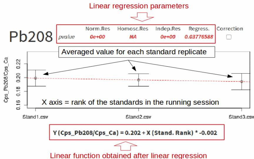
Figure 12: Machine drift verification performed by **elementR**
