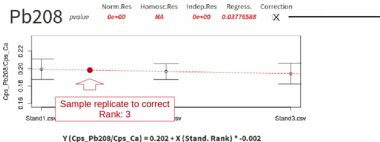
Figure 12: Machine drift correction performed by **elementR** for sample replicate at rank 3
