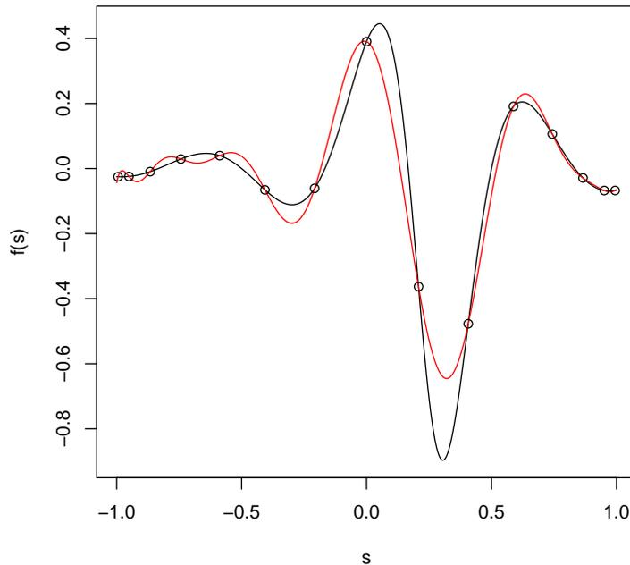
Even though there still are oscillations near the end points, their amplitude will diminish as  $n$  grows. The knots are the locations where the curves intersect.
