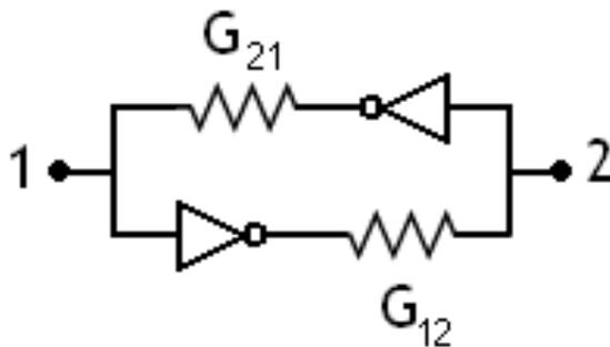
Figure 6: A differential resistor, with diodes set up to enforce a one-way flow of current; if current flows from node 1 to 2, the conductance equals  $G_{12}$  and current only goes through the bottom path; likewise, the conductance is  $G_{21}$  if current flows in that direction.
