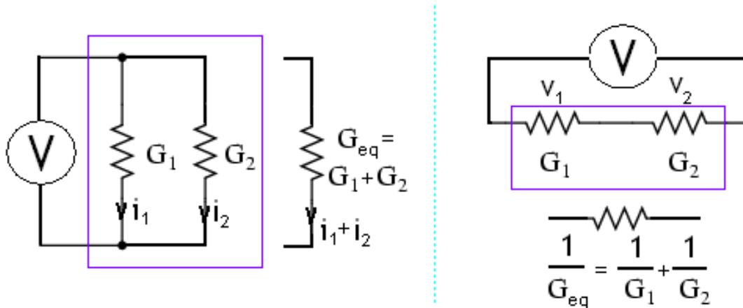
Figure 2: Simple circuits demonstrate compound conductances. In the parallel case on the left, the total conductance is the sum of the respective conductances because the induced current is higher; in the serial case on the right, the total conductance is the reciprocal sum due to the drop in induced current.
