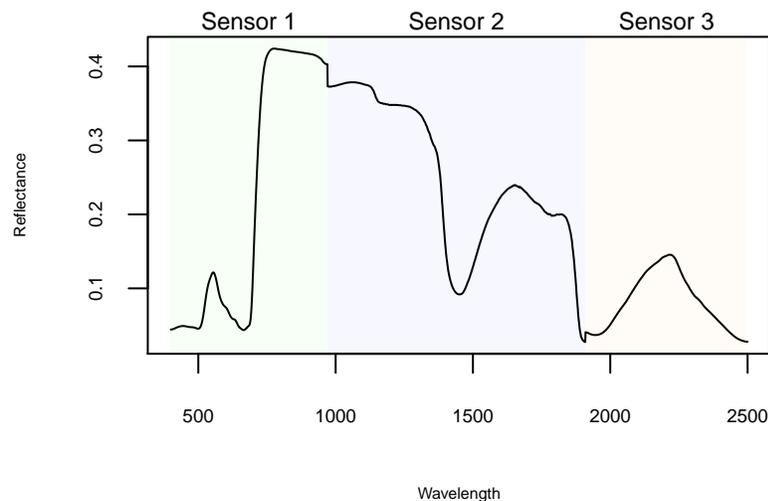
In this case, sensor 1 goes from 400 to 970nm, sensor 2 from 971 to 1909 and sensor 3 from 1910 to 2500. These **boundaries will vary** depending on the individual instrument, so you’ll have to plot and zoom your spectra to figure out where the sensor limits are, which you can do with `plot_interactive`.
