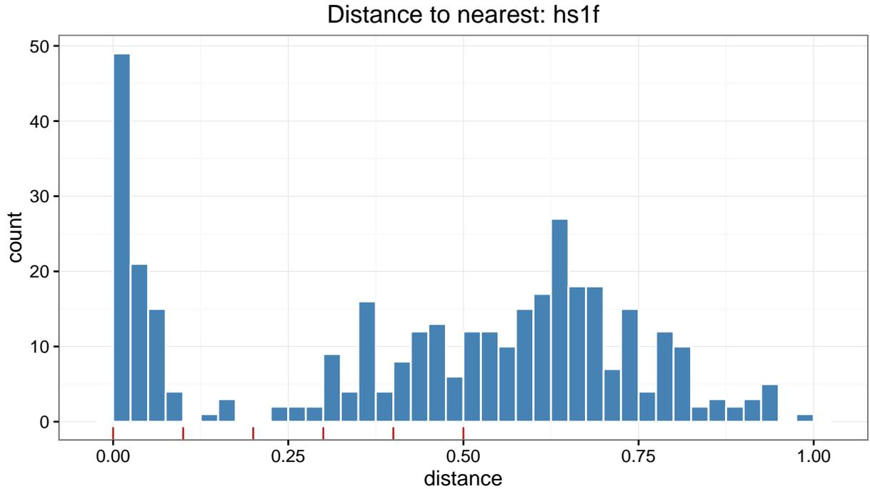
In this example, the length normalized `hs1f` model distance threshold would be set to a value near 0.1.
