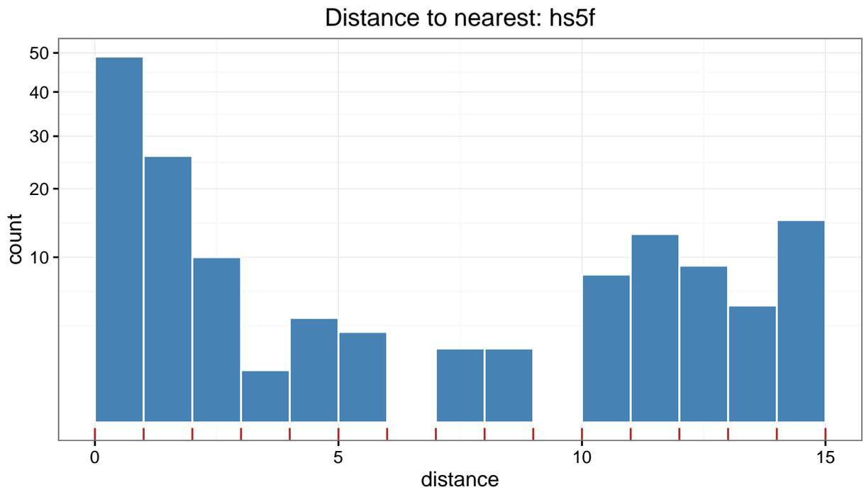
In this example, the unnormalized hs5f model distance threshold would be set to a value near 4.
