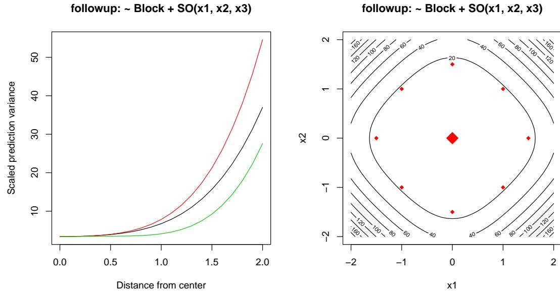
From this we can tell that we can at least augment the design to fit a second-order model. The model includes a block effect to account for the fact that two separately randomized experiments are combined.
