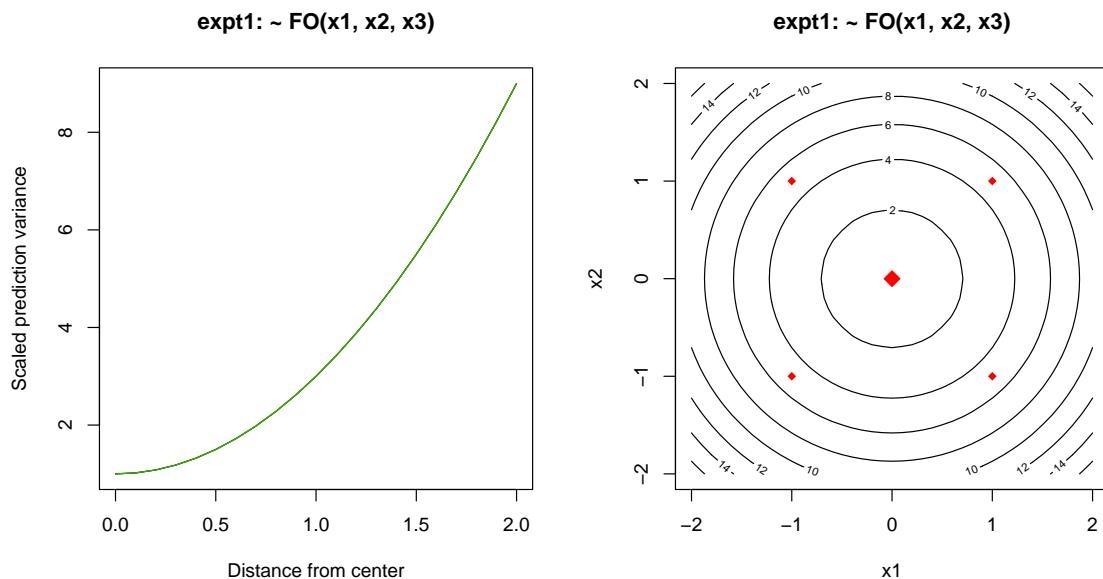
Not surprisingly, the variance increases as we go farther out—that is, estimation is more accurate in the center of the design than in the periphery. This particular design has the same variance profile in all directions: this is called a *rotatable* design.
