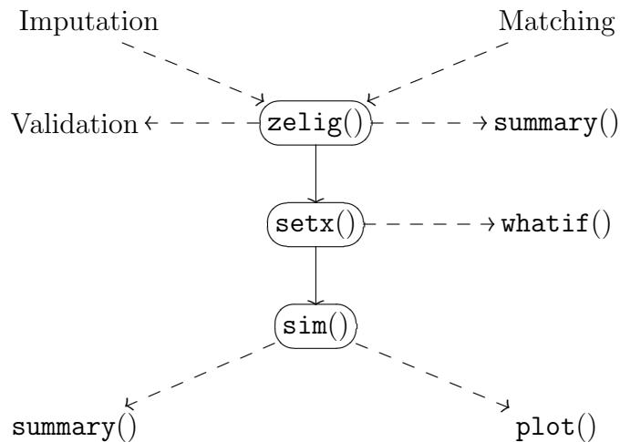
1. Use `zelig()` to run the chosen statistical model on a given data set, with a specific set of variables. For standard likelihood models, for example, this step estimates the coefficients, other model parameters, and a variance-covariance matrix. In addition, you may choose from a variety of options:
