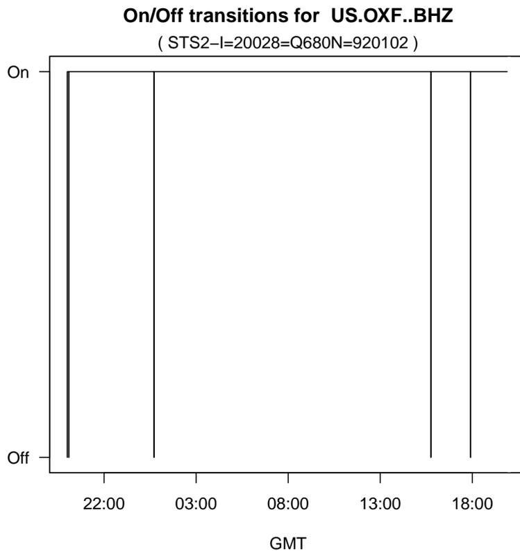
This station had a few minor data dropouts, causing the data to be broken up into several separate signals that the IRISseismic package stores in Trace objects.
