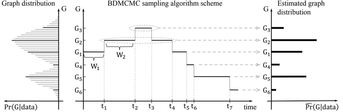
Figure 2: This image visualizes the Algorithm 2. The left side shows the true posterior distribution of the graph. The middle panel presents a continuous time BDMCMC sampling algorithm where  $\{W_1, W_2, \dots\}$  denote waiting times and  $\{t_1, t_2, \dots\}$  denote jumping times. The right side denotes the estimated posterior probability of the graphs in proportion to the total of their waiting times, according to the Rao-Blackwellized estimator.
